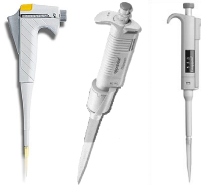
Figure 8 Examples of manual pipettes supplied by Brand GmbH, Eppendorf AG and Thermo Electron Corporation
